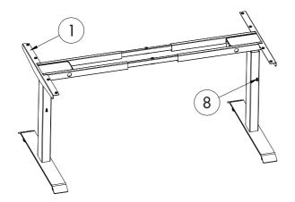
STEP 4: Slide the side bracket (part 1) into the frame end. Insert the two (2) M6\*14 screws (part 8) through the two (2) holes in the bottom of the frame end going into the inserted side bracket (part 1). Using the allen wrench rotate each screw just a few turns. After both M6\*14 screws (part 8) inserted, tighten both screws.
