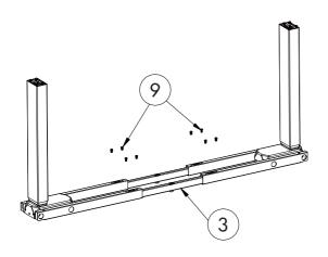
STEP 2: Install the center rail (part 3) with eight (8) M6\*10 screws (part 9). Slide the two (2) center rail (part 3) into the two (2) frame ends ensuring:
