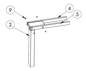
STEP 1: Install the frame left (part 4), frame right (part 5) and lifting column (part 2) with four (4) M6\*10 screws (part 9).
