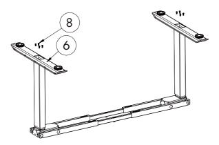
STEP 3: For each leg assembly, attach a foot (part 6) with four (4) M6\*14 screws (part 8) and tighten in a cross-pattern.
