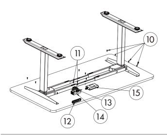
STEP 5: Attach the desk base to the underside of the desktop with ten (10) ST5\*20 wooden screws (part 10).
