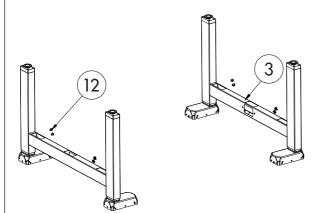
STEP 2: Using the supplied allen wrench, insert four (4) M8\*12 screws (part 12) to fix the beams (part 3) and lifting columns as below picture shows.
