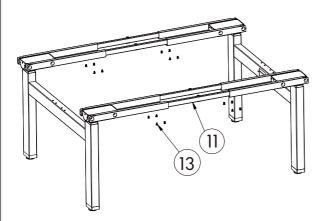
STEP 4: Slide the center rail (part 11) into the two (2) frame ends with eight (8) M6\*10 screws (part 13)ensuring:
