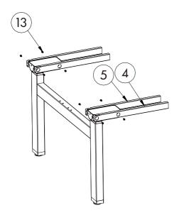
STEP 3: Using two (2) M6\*10 screws (part 13) to fix frame left (part 5) and two (2) M6\*10 screws (part 13) to fix frame right (part 4).
