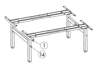
STEP 5: Slide the side bracket (part 1) into the frame end. Insert the two (2) M6\*14 screws (part 14) through the two (2) holes in the bottom of the frame end going into the inserted side bracket (part 1). Using the allen wrench rotate each screw just a few turns. After both M6\*14 screws (part 14) inserted, tighten both screws.
