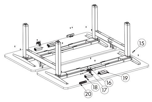
STEP 7: Attach the desk base to the underside of the desktop with ten (10) ST5\*20 wooden screws (part 15). Install the control box (part 19) underside of the desktop with two (2) ST5\*20 wooden screws (part 15). Install the power adapter fixing (part 17) with two (2) ST5\*16 wooden screws (part 16).
