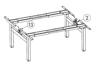
STEP 6: Using four (4) M6\*10 screws (part 13) to fix screen holder (part 2) with frames .
